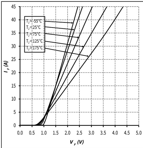
Figure 1. Forward Characteristics
