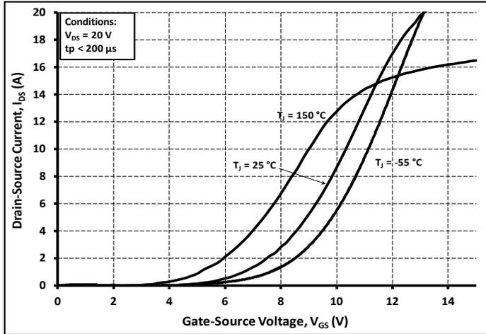
Figure 7. Transfer Characteristic for Various Junction Temperatures
