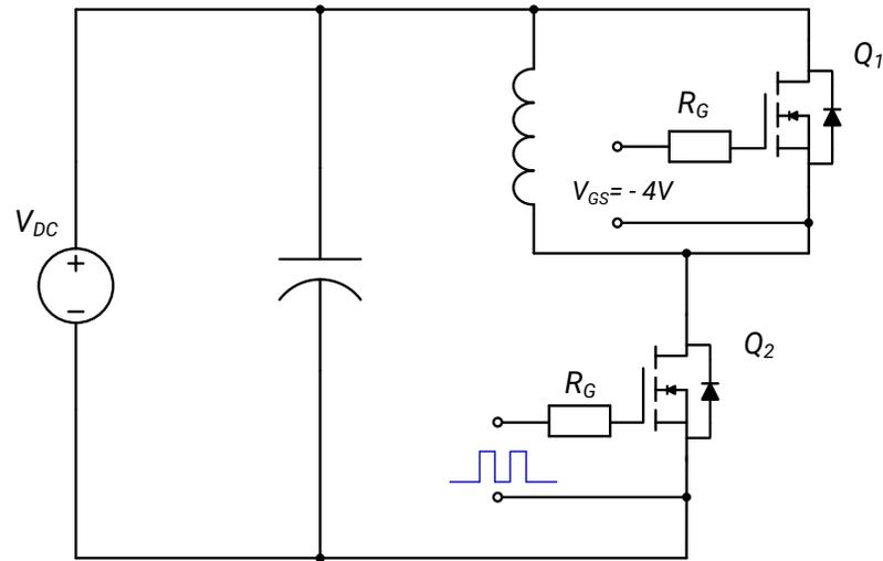
**Figure 29a.** Clamped Inductive Switching Waveform Test Circuit
