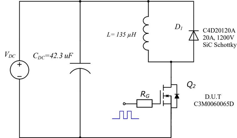
**Figure 27.** Clamped Inductive Switching Waveform Test Circuit
