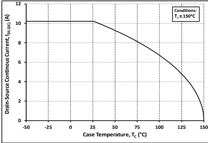
Figure 19. Continuous Drain Current Derating vs Case Temperature
