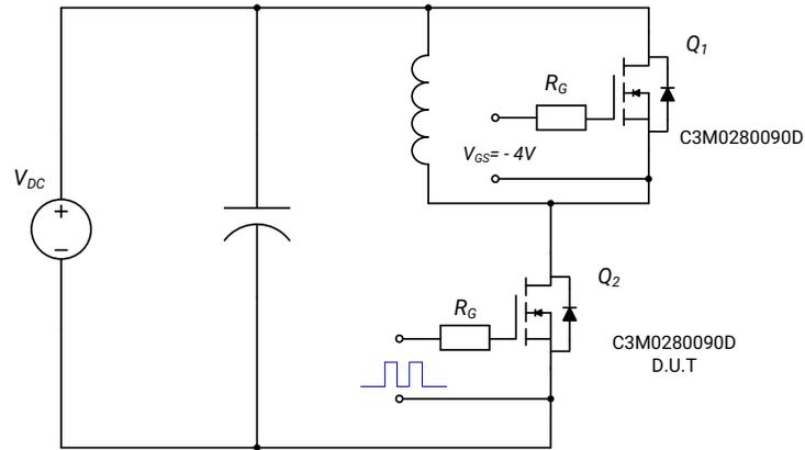
**Figure 29.** Clamped Inductive Switching Test Circuit
