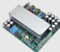
6.6 kW High Power Density Bi-Directional EV On-Board Charger CRD-06600FF065N-K
