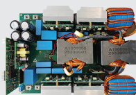
22 kW Bi-Directional CLLC Utilizing IMS Board
