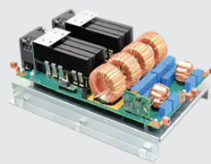
60 kW INTERLEAVED BOOST CONVERTER CRD-60DD12N
