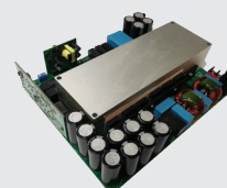
6.6 kW High Power Density Bi-directional EV ON-Board Charger
