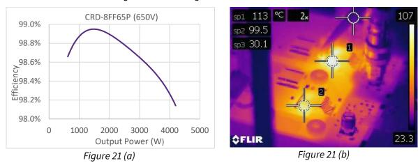
Figure 23 (a): Synchronous boost converter efficiency, Figure 21 (b): Synchronous boost converter thermal scan at 4200 W
