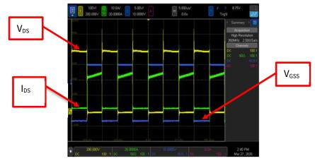
Figure 22: Switching waveforms of boost converter
