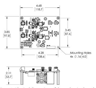
Figure 2: Physical dimensions of the evaluation board
