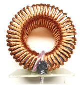
Figure 24: Synchronous boost inductor
