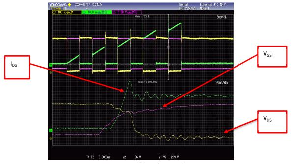
Figure 27: Double pulse waveform
