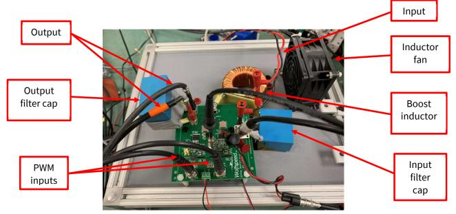
Figure 21: Synchronous boost converter setup
