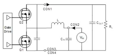
Figure 19: Synchronous boost converter schematic
