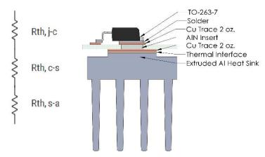
Figure 18: Thermal management stack up
