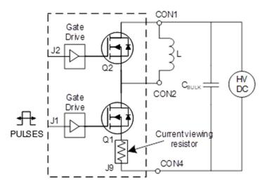
Figure 25: Clamped inductive switching measurement circuit
