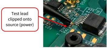
Figure 15: Test lead clipped on the source (power)
