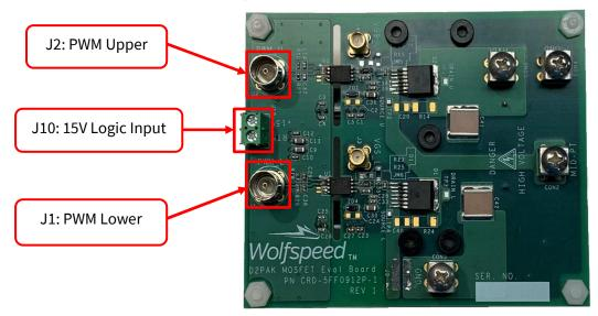
Figure 14: Low-voltage input connectors
