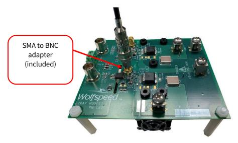
Figure 16: SMA to BNC adapter and X10 passive probe
