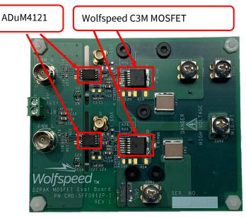
Figure 11: Gate driver and MOSFET locations
