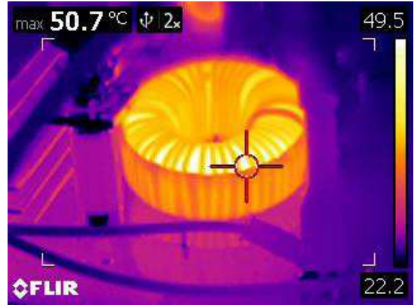
Figure 19: Thermal scan of Inductor (1200V)
